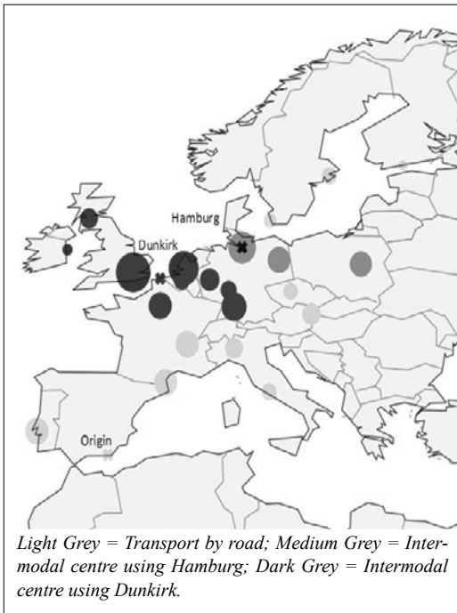
Figure 5 - Possible intermodal strategy (O6 agile). Metric tonnes transported.
